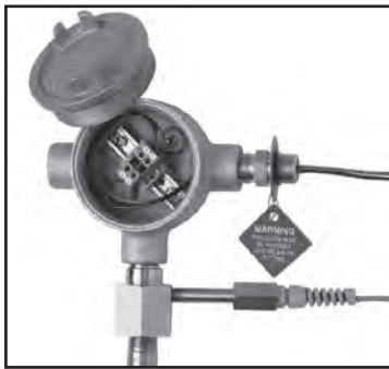
Secondary Process Sealing Fittings. Cooper Crouse-Hinds has invented the first CSA approved, field installed, pressure rated process seal which stops both gases and liquids, under pressure, from migrating through conduit and individual conductors.
